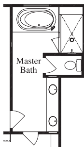
Drop-In Tub with Large Mudset Shower with Seat & Niche at Master Bath
